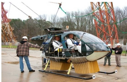
Figure 1. NASA's helicopter drop test [1].
